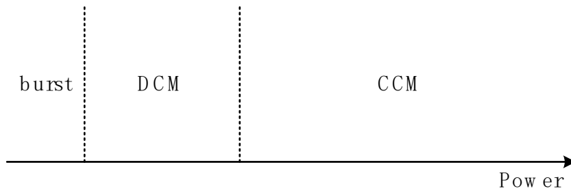
Figure 5 Operating Mode of OSU1010A
